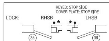
\* Indicates lock mounting/access plate side.
