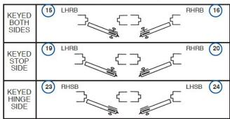
1-1/4" projection required with stop-side mounting.
