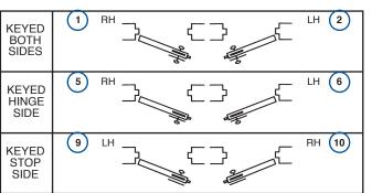
1-1/4" projection required with stop-side mounting.
