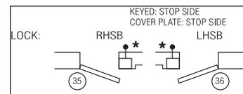
\* Indicates lock mounting/access plate side.
